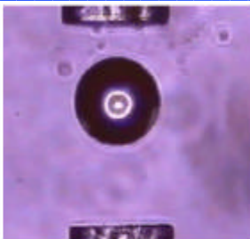
Fig. 2. A 100 micron polymer sphere trapped in a fibre optical light force trap, viewed from below. The fibre trap uses 62.5/125µm (core size/ cladding size) multimode fibre, a trapping power of 800mW in each fibre arm and a fibre separation of 240µm.
