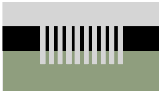
Figure 2 Side view of a photonic-crystal slab. The light gray region is air, the black region is the core layer, and the gray-green region is the substrate. Air holes have been etched down to the substrate.
