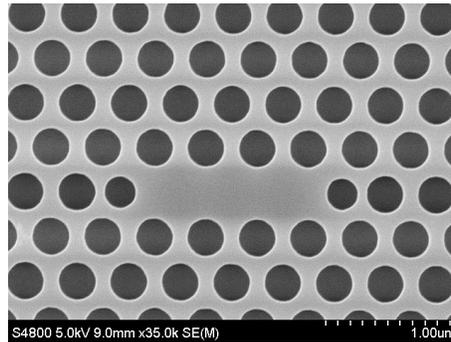
Fig. 9. SEM micrograph of a L3 PhC cavity.
