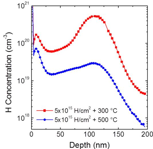
Fig. 7. H chemical profiles, as obtained by SIMS, of a SOI implanted with  $5 \times 10^{15}$  H/cm<sup>2</sup> and annealed at 350 °C (red squares and line) and at 500 °C (blue circles and line).
