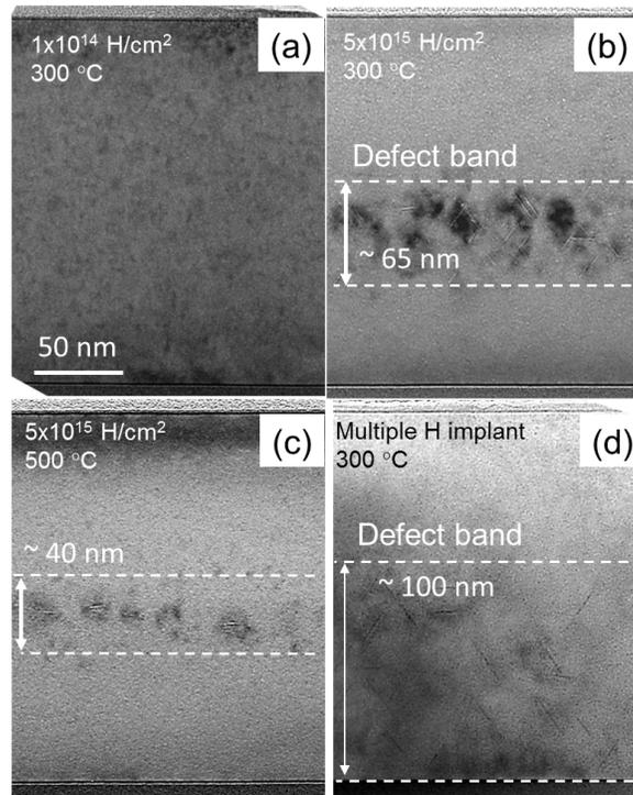
Fig. 6. Cross sectional TEM images of SOI implanted with 8 keV H to a dose of  $1 \times 10^{14}$  H/cm<sup>2</sup> and annealed at 300 °C (a), to a dose of  $5 \times 10^{15}$  H/cm<sup>2</sup> and annealed at 300 °C (b) and 500 °C (c). The CS TEM image of a SOI sample after multiple H implants and annealed at 300 °C is reported in (d).
