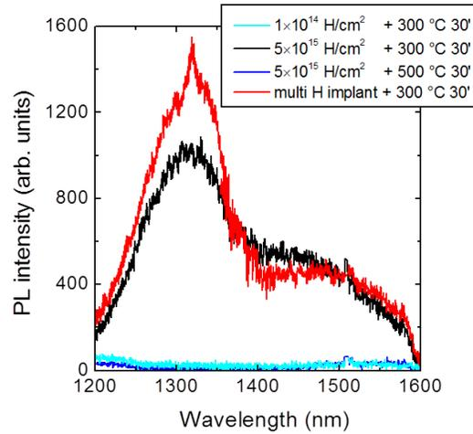
Fig. 8. Photoluminescence spectra of SOI samples implanted with a dose of  $1 \times 10^{14}$  H/cm<sup>2</sup> at 8 keV and annealed at 300 °C (light blue line), a dose of  $5 \times 10^{15}$  H/cm<sup>2</sup> and annealed at 300 °C (black line) and 500 °C (blue line). The PL spectrum of the SOI sample after multiple H implants and annealed at 300 °C is also reported (red line).
