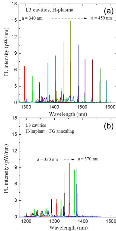
Fig. 10. Photoluminescence spectra of L3 PhC nanocavities having different lattice constant  $a$ , (a) H-plasma treated PhC cavities (b) H-implanted PhC cavities followed by thermal treatment in forming gas.
