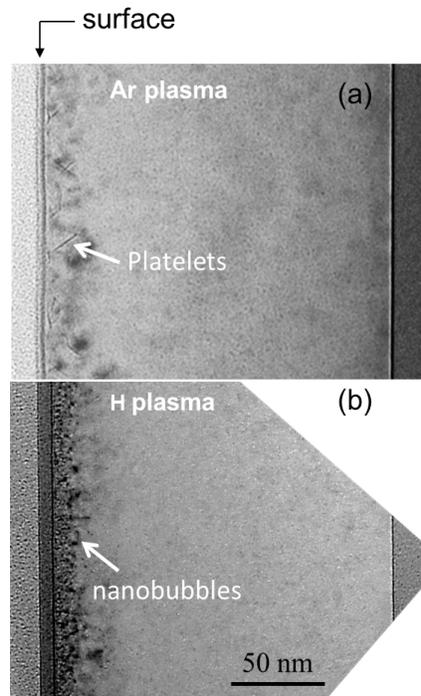
Fig. 1. Cross sectional TEM of SOI after the exposure to a 40 W plasma treatment for 30 min in Ar (a) and H<sub>2</sub> (b).
