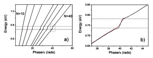
FIG. 4. (Color online) (a) Absolute phase delay for samples having an increasing number of layers. Left to right: 10, 15, 20, 28, 31, 35, and 40 layers. (b) Detail of the results for the sample 40 layers thick in the vicinity of the pseudogap. Experimental data appear as red lines and theoretical calculations as black ones. Horizontal dashed lines indicate the edges of the L pseudogap as extracted from band calculations.
