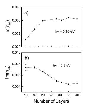
FIG. 7. Evolution of the imaginary part of the effective refractive index as a function of the number of layers for a frequency contained within the gap (a) and outside of it (b).
