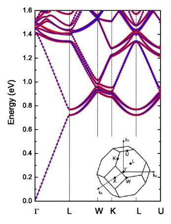
FIG. 1. (Color online) Red circles: photonic bands of a polystyrene opal consisting of close-packed spheres of diameter b=708 nm and dielectric constant  $\varepsilon=2.455$  in air. Blue lines: photonic bands of the same fcc structure when each dielectric sphere is replaced by five cylinders oriented along the [111] direction (Ref. 22). Inset: Brillouin zone of the fcc lattice.
