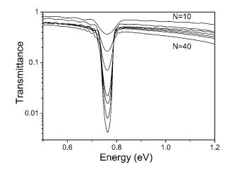
FIG. 2. Transmittance spectra in a logarithmic scale for samples made from spheres of 705 nm nominal diameter, having different thickness. Top to bottom: 10, 15, 20, 28, 31, 35, and 40 layers.
