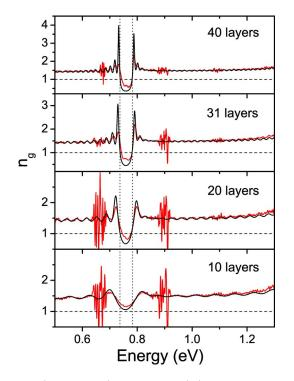
FIG. 8. (Color online) Group index  $(n_g)$  for samples with increasing number of layers. Top to bottom: 40, 31, 20, and 10 layers. Horizontal dashed lines indicate the limit of superluminal velocity  $v_g = c$ . Vertical dotted lines indicate the pseudogap edges predicted by calculated bands. Experimental data appear as red lines and theoretical calculations as black ones.
