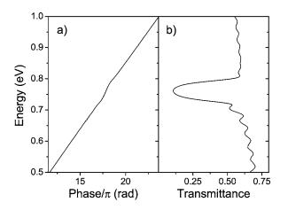
FIG. 3. (a) Phase delay introduced by a sample 18 layers thick made of spheres of diameter 705 nm. (b) Transmittance collected from the same spot on the sample as the phase delay.
