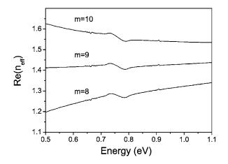
FIG. 6. Effective refractive index estimated for a 20 layers thick sample after subtracting three consecutive multiples of  $2\pi$  from the measured phase (see text). The data in the middle correspond to the multiple obtained by linearly extrapolating the phase delay in the low energy region. The top/bottom curve corresponds to a multiple larger or smaller by one.
