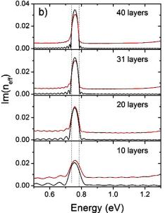
FIG. 5. (Color online) Real (a) and imaginary (b) parts of the effective refractive index estimated from the absolute phase and transmittance, respectively, for different sample thicknesses: top to bottom 40, 31, 20, and 10 layers. Vertical dashed lines indicate the edges of the L pseudogap as extracted from band calculations. All samples are made of spheres with 705 nm nominal diameter. Experimental data appear as red lines and theoretical calculations as black ones.
