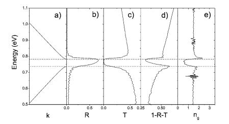
FIG. 9. (a) Band structure for a polystyrene opal along the  $\Gamma L$  direction. (b) Reflectance, (c) transmittance, and (d) diffuse intensity for a 42 layers thick sample. (e) Group index for a 40 layers thick sample.
