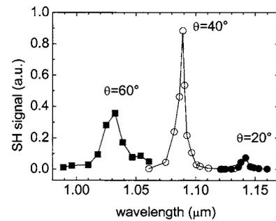
FIG. 3. Experimental results for the transmitted second-harmonic signal as a function of the pump wavelength in the resonance region, for  $p$ -polarized pump and harmonic waves, at three different values of the incidence angle.
