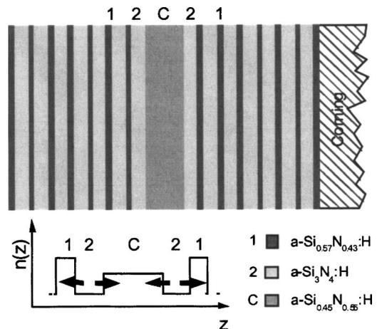
FIG. 1. Upper panel: layout of the microcavity structure, made of a defect layer "c" embedded between two dielectric mirrors made of layers "1" and "2." Lower panel: schematic profile of the refractive index. The arrows at the interfaces denote the direction from low to high refractive index, determining the sign of the  $\chi^{(2)}$  components.
