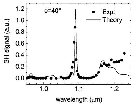
FIG. 4. Transmitted second-harmonic signal as a function of the pump wavelength, for *p*-polarized pump and harmonic waves, at an incidence angle of 40°.
