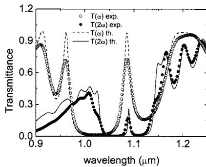
FIG. 2. Linear transmittance for  $p$ -polarized light at an incidence angle of  $40^\circ$ , in the spectral region of the pump wave (open dots and dashed line) and of the second-harmonic wave (full dots and solid line), as a function of the pump wavelength. Points: experimental results. Lines: theory.
