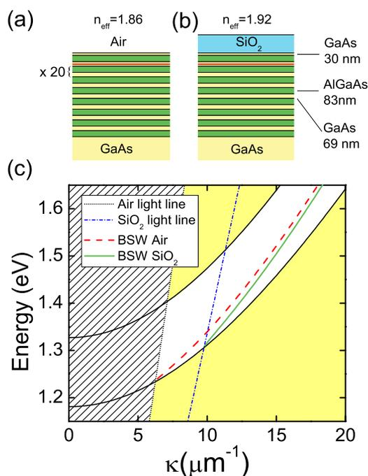
FIG. 1. (Color online) Scheme of the structures under investigation: (a) multilayer stack supporting in-plane propagating Bloch surface modes with the air cladding (b) same multilayer with a 500 nm silica layer in the cladding. (c) Calculated mode dispersion of BSWs for the structure in (a) (dashed line) and (b) (solid line), as a function of the planar momentum,  $\kappa$ ; The air and silica light lines and the Bragg gap of the multilayer are indicated.
