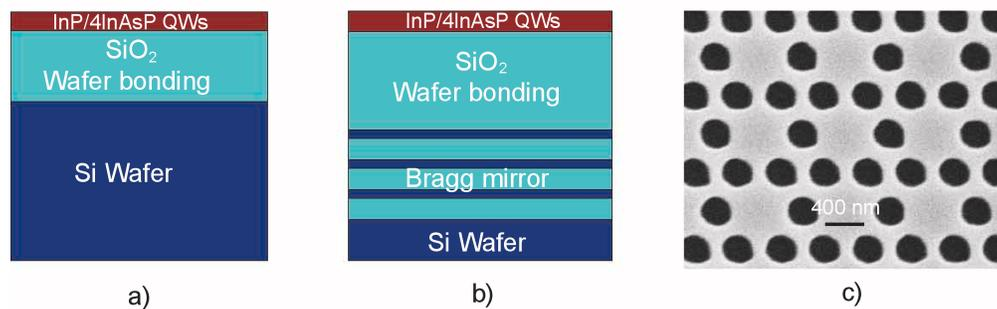
Fig. 1. Layout of the transversal section of the fabricated structures. (a) InP/InAsP layer epitaxy bonded to a Si wafer. (b) InP/InAsP layer epitaxy bonded to a Bragg reflector on top of the Si wafer. (c) Scanning electron microscopy (SEM) image of the fabricated structure with Bragg mirror.
