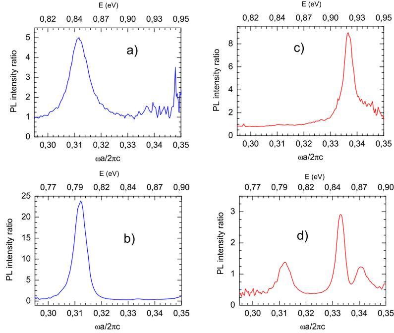
Fig. 3. Normalized PL spectra along the direction  $\Gamma$ -X1, for the sample without Bragg (a,c) and for the sample with Bragg reflector (b,d) at angle  $\theta = 25^\circ$ . Blue line for even ( $\sigma_{kz} = +1$ ) or p-polarization, red line for odd ( $\sigma_{kz} = -1$ ) or s-polarization with respect to a vertical mirror plane.
