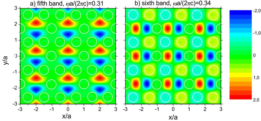
Fig. 4. Real part of magnetic field component  $H_z$  at the  $\Gamma$  point for the photonic modes corresponding to the resonant structures in Fig. 3(a) at  $\omega a/(2\pi c) = 0.31$  (fifth band) and in Fig. 3(c) at  $\omega a/(2\pi c) = 0.337$  (sixth band).
